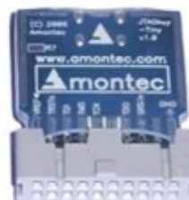
Figure 2-2: JTAGkey "Tiny" device from Amontec
